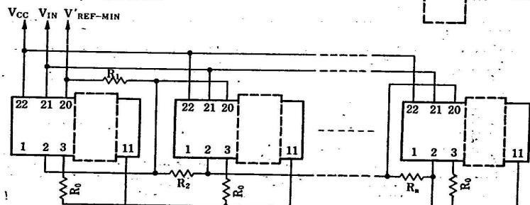
$$\frac{V'_{REF-MAX} - V'_{REF-MIN}}{\sum R_i} > (n-1) \times 100 \text{ } (\mu\text{A}) \quad (i=1,2,\dots,n)$$
