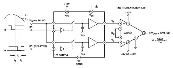
Figure 23. Time Delta Sample-and-Difference Measurement
