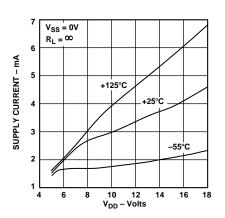
Figure 11. Supply Current vs. V<sub>DD</sub>
