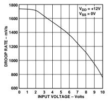
Figure 3. Droop Rate vs. Input Voltage ( $T_A = +125^{\circ}C$ )
