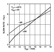
Figure 6. Slew Rate vs. V<sub>DD</sub>
