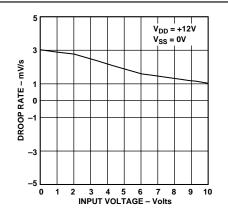
Figure 2. Droop Rate vs. Input Voltage ( $T_A = +25^{\circ}C$ )
