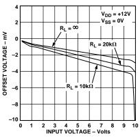
Figure 9. Offset Voltage vs. Input Voltage ( $T_A = -55^{\circ}C$ )
