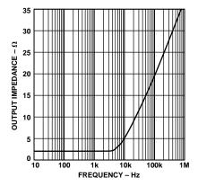
Figure 14. Output Impedance vs. Frequency
