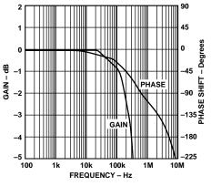
Figure 13. Gain, Phase Shift vs. Frequency
