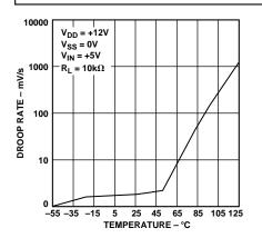
Figure 1. Droop Rate vs. Temperature
