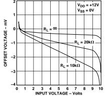
Figure 7. Offset Voltage vs. Input Voltage ( $T_A = +25^{\circ}C$ )
