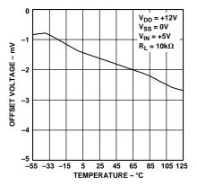
Figure 10. Offset Voltage vs. Temperature
