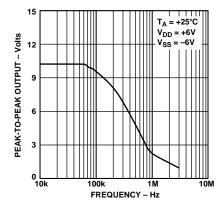
Figure 15. Maximum Output Voltage vs. Frequency
