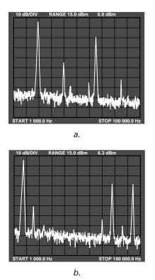
Figure 16. Spectral Response at a Sampling Frequency of 86 kHz. Photo (a) Shows a 20 kHz Carrier Frequency and Photo (b) Shows an 8 kHz Frequency.
