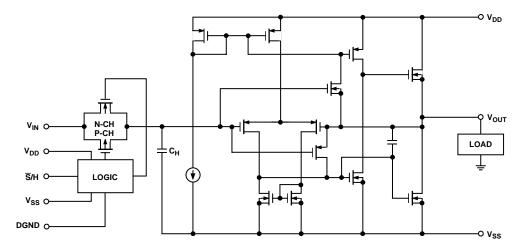
Figure 27. Simplified Schematic of One Channel
