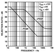
Figure 12. Sample Mode Power Supply Rejection
