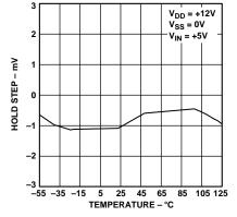
Figure 5. Hold Step vs. Temperature
