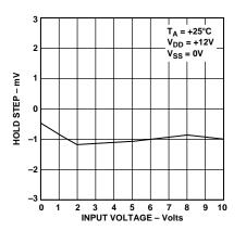
Figure 4. Hold Step vs. Input Voltage
