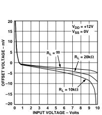
Figure 8. Offset Voltage vs. Input Voltage ( $T_A = +125^{\circ}C$ )
