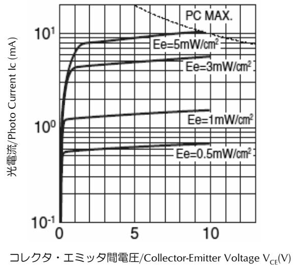
$E_e = 1 \text{ mW}/\text{cm}^2$ を基準とする/It is based on  $E_e = 1 \text{ mW}/\text{cm}^2$ .
