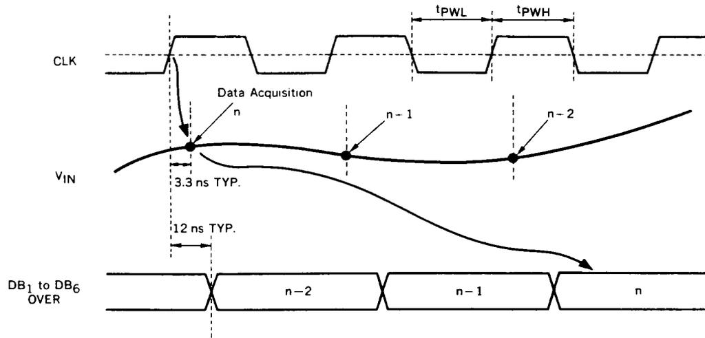
Analog signal is sampled with sampling clock and after the acquisition time (3.3 ns TYP.) started to be sampled. And converted data will be out after 2 sampling clock synchronized with the rise edge of sampling clock. Delay time from the rise edge of sampling clock is typically 12 ns.
