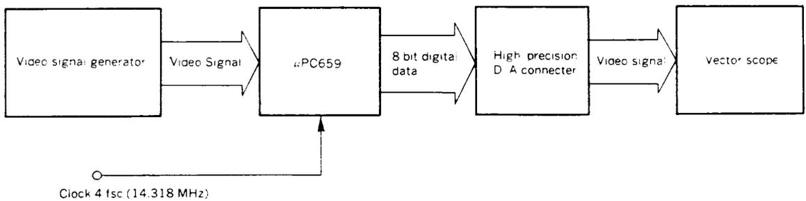
The video signal from the video signal generator is 40 IRE Ramp signal.
