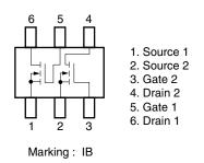
**Remark** The diode connected between the gate and source of the transistor serves as a protector against ESD. When this device actually used, an additional protection circuit is externally required if a voltage exceeding the rated voltage may be applied to this device.
